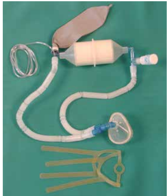
DAN experts developed this remote emergency oxygen (REMO 2 ) surface oxygen rebreather for first-aid use (Pollock and Natoli 2007).
