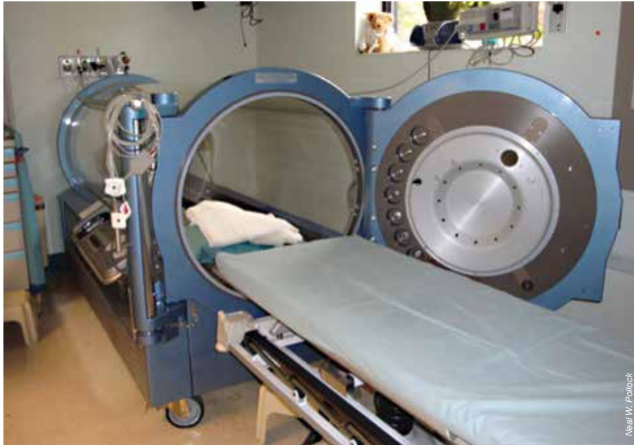
This is a monoplace hyperbaric chamber — able to hold a single patient, without any inside support personnel, or “tenders.”
